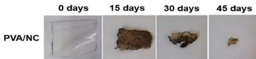
Figure 10. Evaluation of the visual appearance of the PVA/NC film after the biodegradation test.
