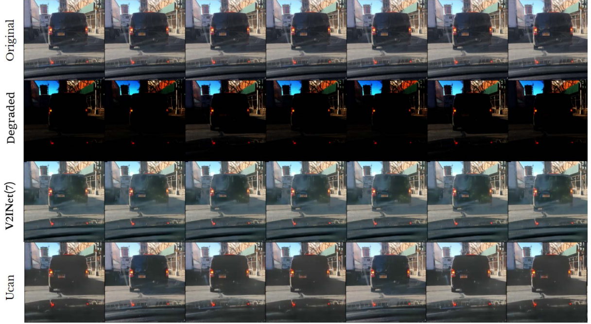
Figure 7: Comparison showing the original video, the synthetically underexposed video, and the outputs from the V2INet (ours) and the UCan [34] networks. It is possible to observe a higher variation in the exposure levels of the frames restored by the UCan method (last row), particularly in the car dashboard panel. In the other hand, the sequence restored by our V2INet method presents more coherent exposure along the sequence.
