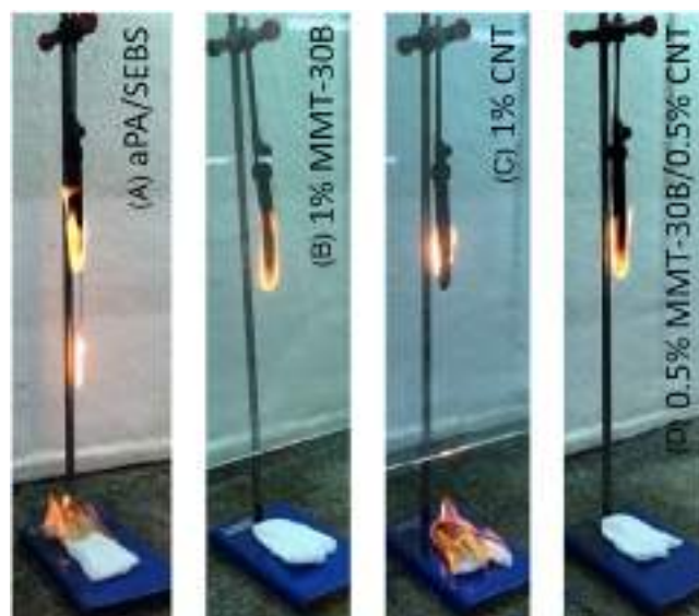
FIGURE 5 Flammability test photos for the blend (A) and nanocomposites with MMT-30B and CNT (B)–(D)
